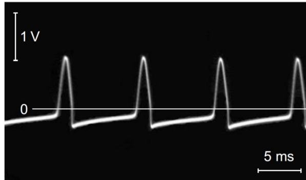
FIG. 5.7. Typical train of spikes V_C(t) from the analogue circuit without control.
