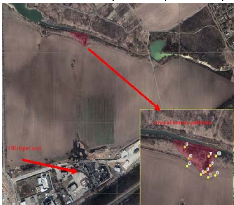
Figure 3. Documented contamination of the geological environment in the area of the destroyed oil depot based on drilling results
