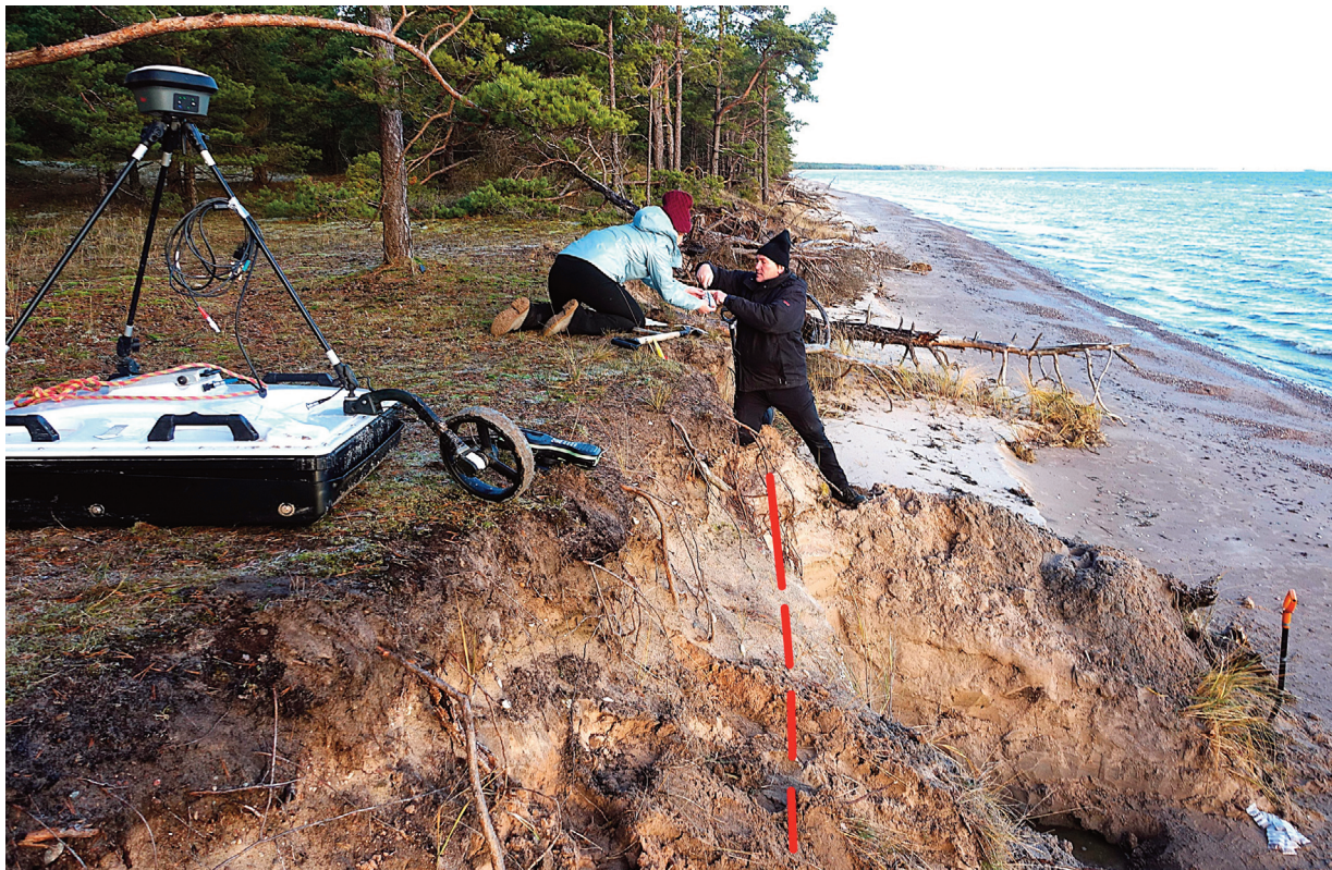
Fig. 3. Setting of the master outcrop (the sea-facing profile, marked with a red dashed line, is partly obscured); GPR instrument shown on the left. Fallen trees in the background indicate recent scarp erosion. Photo by Ü. Suursaar, 4 December 2024.
