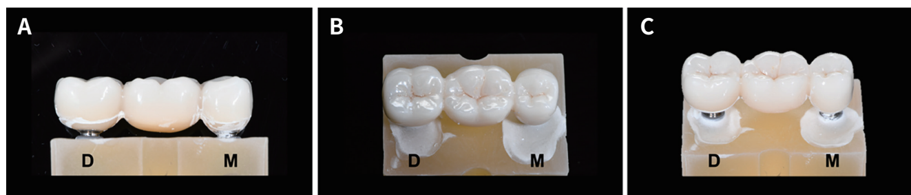
Fig. 2. Experimental model preparation. (A) Overview of the cemented FDP on mesial (M) and distal (D) implants with engaging abutments in the 100-µm vertical misfit simulation. (B) Close-up view of the mesial (M) abutment. (C) Close-up view of the distal (D) abutment.
