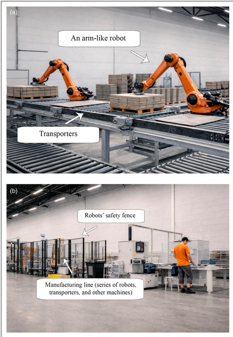
Figure 1. (a) Illustration of arm-like robots in the furniture manufacturing industry 3 (b) Illustration of a robotic manufacturing line in the furniture industry 4
