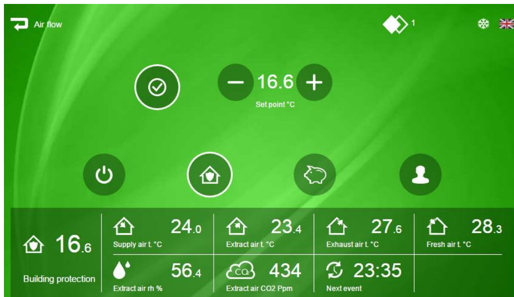
Figure 2. Current air handling unit control user interface
