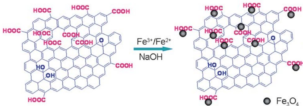
Fig. 11. Magnetic graphene oxide synthesis
