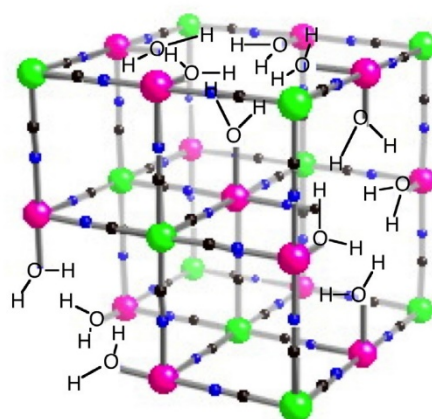
Fig. 7. Structure of Prussian blue (Bhatt et al., 2012)
