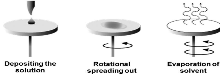
Fig. 8. Spin coating processes of thin-films [20].
