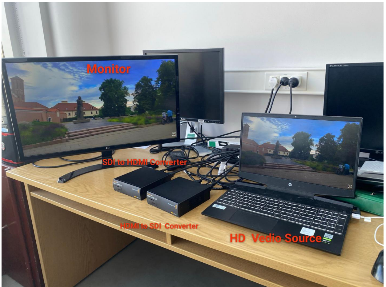
Figure 2.1.1. Conversion and testing of HDMI and SDI
