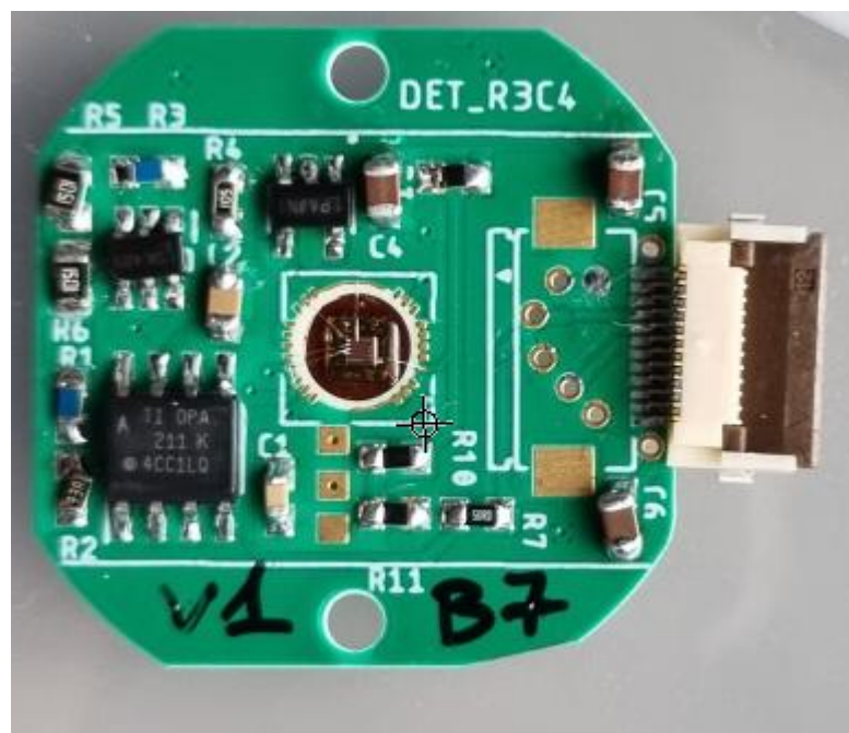
Fig. 18. First step amplifier fully assembled and detector chip contacts bonded to the PCB.
