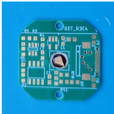
Fig. 16. PCB with gold-plated silica wafer glued in the middle.
