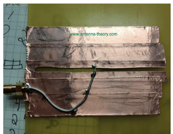
Figure 1: Basic structure and practical implementation of a vivaldi antenna
