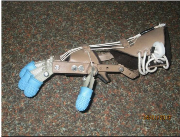
Figure 3: First ever 3DP prostheses "Robohand"
