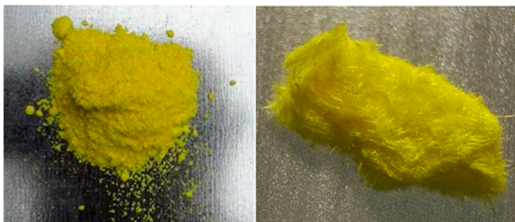
Figure 1. A sample of crystals of 3-picrylamino-1 H -1,2,4-triazole after crystallization at 1\times (left) and 50\times (right) magnifications using a digital microscope.
