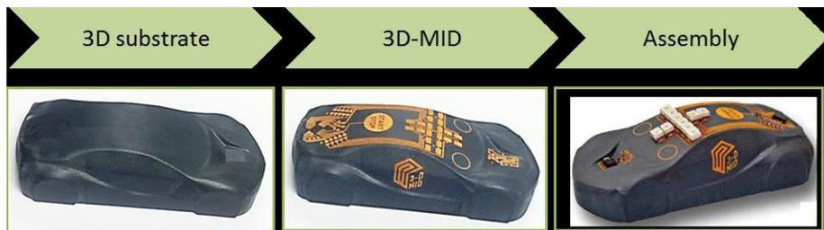
Figure 1. The principle of MID technology [19].
