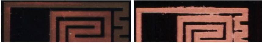
*Figure 35. Examples of underplating (left) and overplating (right) using various regimes of the SSAIL process.*
