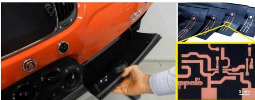
Figure 66. Conductive traces for the FIAT gloves box cover touch button demonstrator [11].
