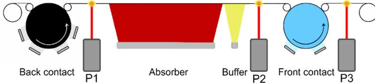
**Fig. 14.** Schematics of the roll-to-roll-based production of CIGS thin-film solar cells. Figure adapted from [59].
