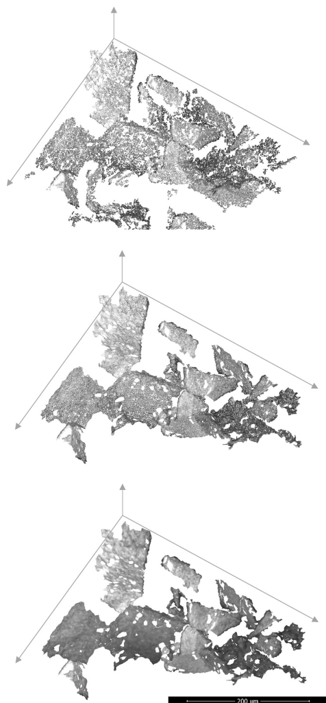
Fig. 6. 3D CHAp synthesized with tartaric acid (TA:Ca = 1) surface reconstruction steps, from point cloud (top), to mesh (middle) and surface (bottom).
