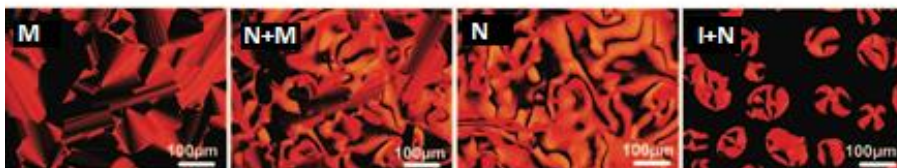
Fig 2.3.1 Phase diagram and polarizing microscope textures of SSY water solutions (adapted from Park et al. [69]) Note the close similarity with Horowitz et al. data [66]
