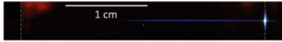
Fig. 3 Side view photography of the blue fluorescence of fused silica induced by a near infrared laser pulse at 1.9 \mu\text{m} with 8 \mu\text{J} energy. The laser pulse is focused on a 70 \mu\text{m} spot (FWHM) at the entrance surface of the 3 cm thick sample. Vertical dash-dotted lines indicate the positions of the entrance and exit surfaces of the sample. Adapted from [5]
