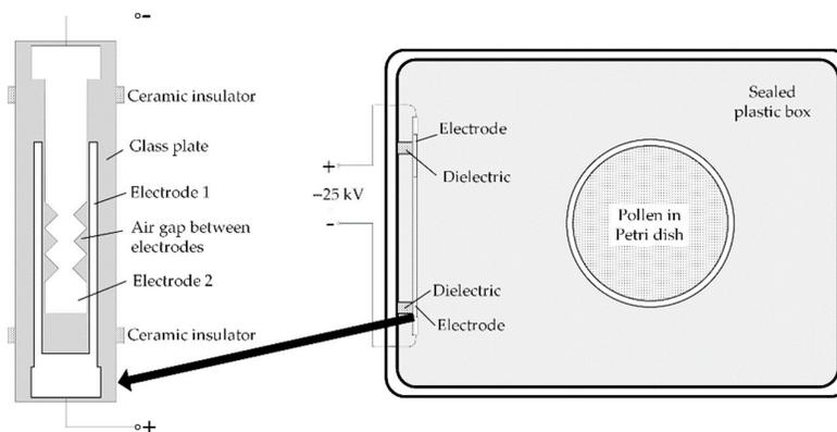
**Figure 1.** Pollen sample exposure to O<sub>3</sub> experimental set-up and high voltage electrical discharge system configuration.
