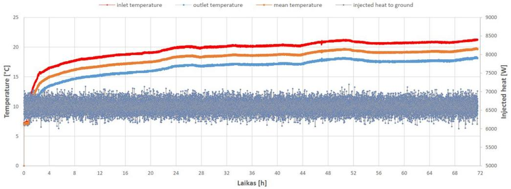
Figure 13 Temperature dynamics of inlet, outlet fluid and injected heat energy
