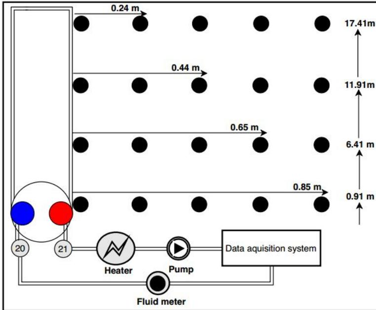
Figure 4 Measurement points schema in one part of the sandbox [23]
