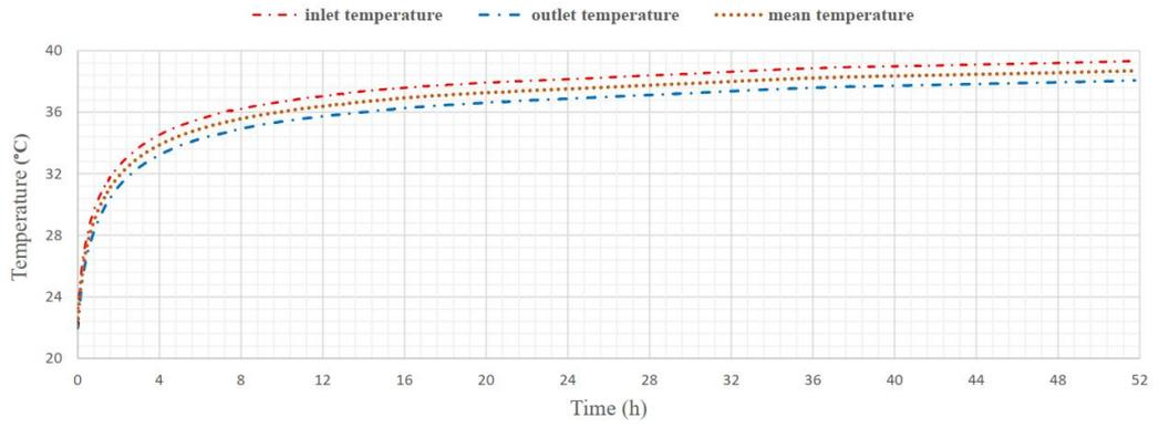
Figure 14 Fluid temperature dynamics
