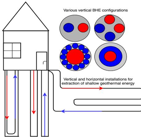
Figure 1 Various BHE configurations
