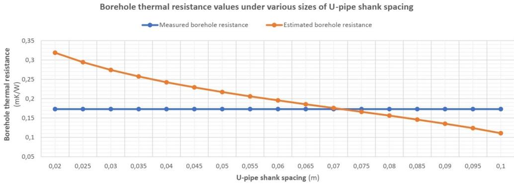
Figure 11 The U-pipe shank spacing value effects on  $R_b$  Indriulionis (2019)[23]
