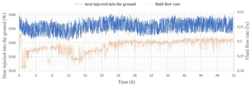
Figure 15 Fluid flow rate and injected heat energy
