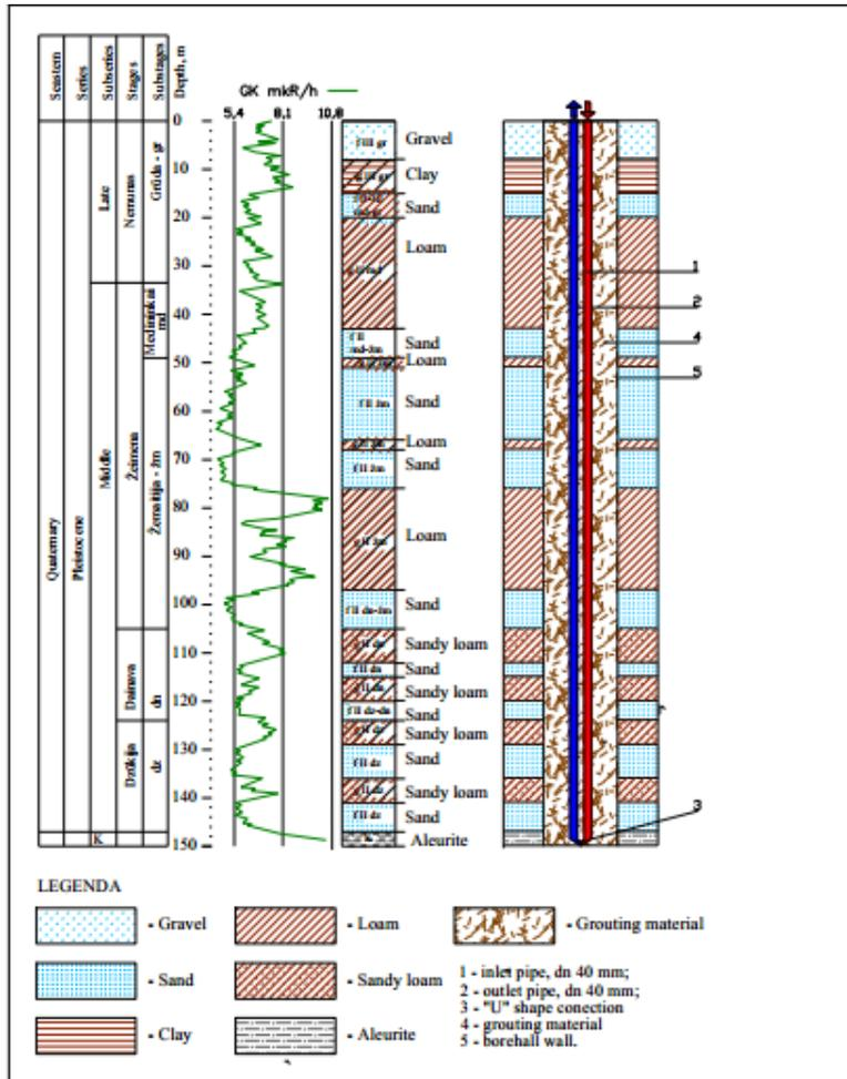
Figure 3 Vertical borehole heat exchanger in the Quaternary sediments [22]
