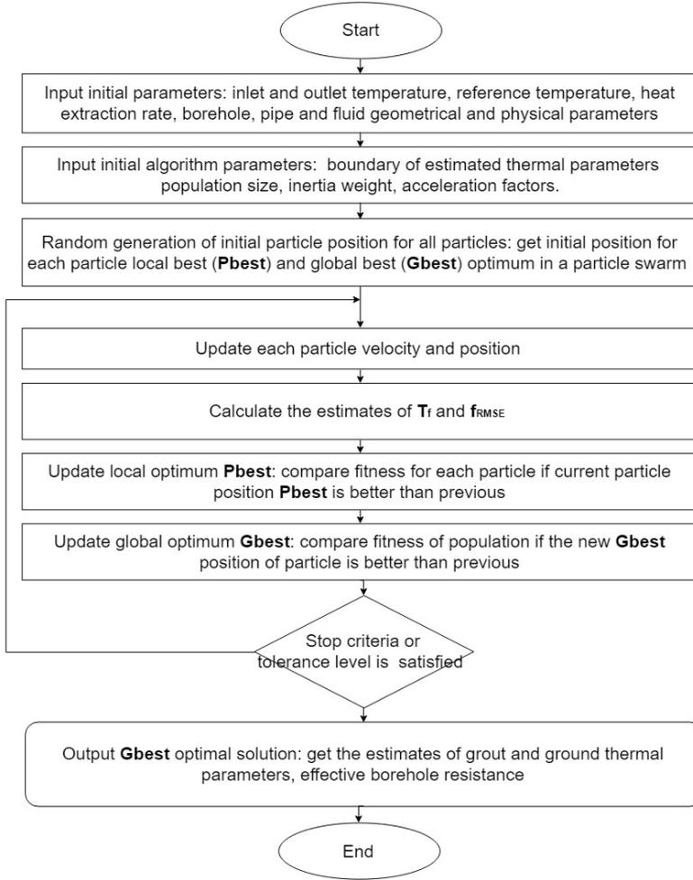
Figure 7 The thermal parameters estimation procedure Indriulionis (2019)[23]
