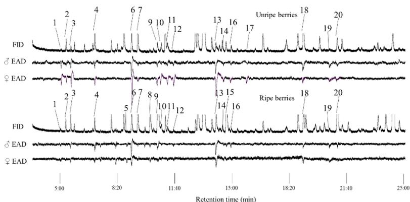
Figure 6. Flame-ionization (FID) and electroantennogram detector (EAD) recordings of antennal responses of *Rhagoletis batava* male and female fruit flies to VOCs of unripe and ripe sea buckthorn berries. Names of the compounds indicated by numbers are presented in Table 1.
