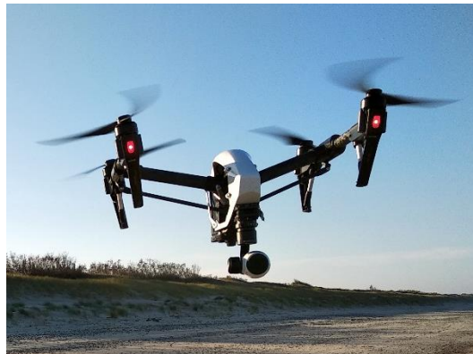
Fig 2. DJI INSPIRE 1 UAV system used in this study.
