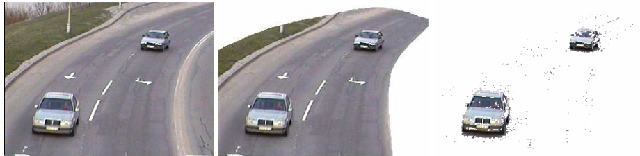
Fig. 1. Before masking. Fig. 2. After masking. Fig. 3. After subtraction.
