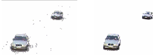
Fig. 4. Blobs filtering. Fig. 5. After 3 \times 3 median filtering.
