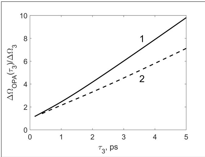
**Fig. 7.** Dependence of OPA bandwidth normalized to pump pulse bandwidth on pump pulse duration.  $z/L_n = 5$  (1),  $z/L_n = 10$  (2).
