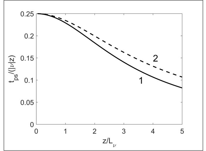
**Fig. 2.** The time delay between signal and pump pulses.  $z/L_n = 5$  (1),  $z/L_n = 10$  (2).
