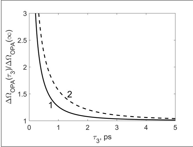
**Fig. 6.** Dependence of OPA bandwidth on pump pulse duration.  $z/L_n = 5$  (1),  $z/L_n = 10$  (2).
