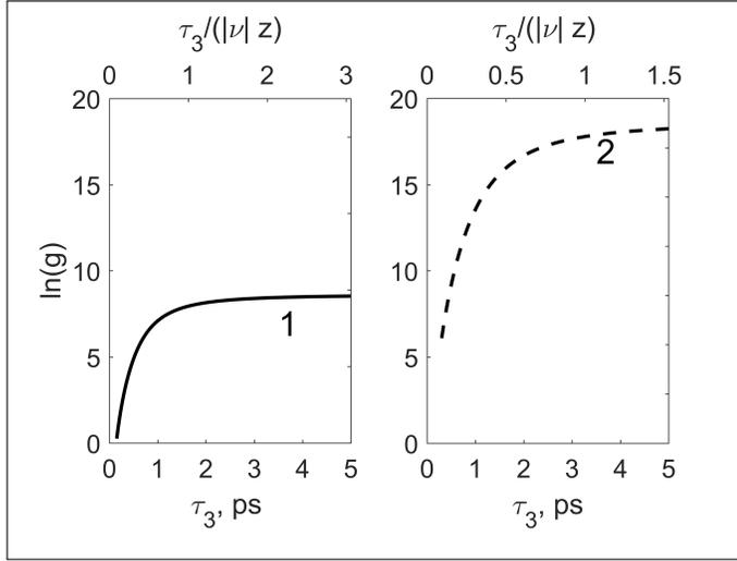
**Fig. 4.** Dependence of signal pulse gain on pump pulse duration  $\tau_3$  (bottom axis) and ratio  $\tau_3/(|\nu|z)$  (top axis).  $z/L_n = 5$  (1),  $z/L_n = 10$  (2).
