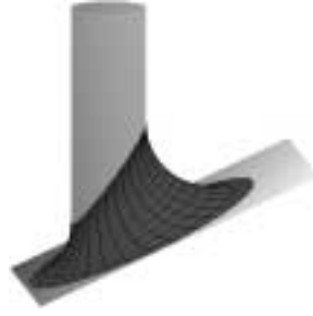
Figure 7. A part of the pipe surface smoothly connecting the cylinder and the plane.
