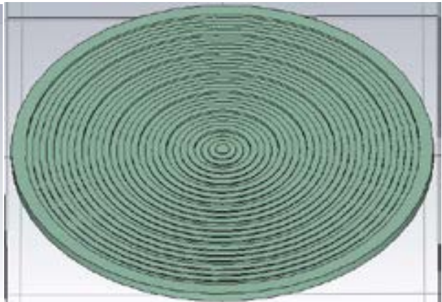
Fig. 2. BZP with a quantization level of N=4 and number of zones Z=7 .
