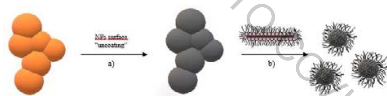
Fig.1. \beta\text{-NaGdF}_4:\text{Yb}^{3+}/\text{Er}^{3+} surface modification steps: removal of hydrophobic oleic acid ligands (a); nanoparticle surface modification using anionic brush-type p(MAA- stat -PEO 9 MEMA) polyelectrolytes (b).
