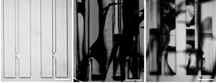
Figure 2.17: Glass cantilevers before immersing the structure with polymer ( left ). The same structure after the polymer heating step: generated cracks into the volume of SZ5050 ( center ) and SZ4060 ( right ) photopolymers. Scale bar, 500 \mu\text{m} .
