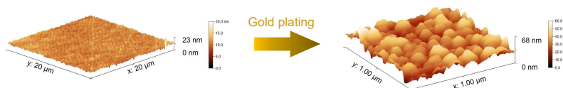
Picture 1. AFM image of 0.25 \mu\text{m} polished Si prism surface (left) covered with gold by electroless plating (right).
