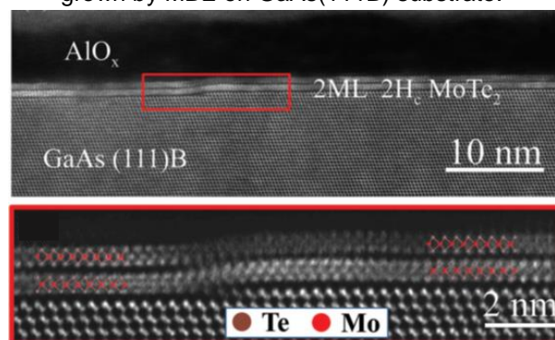
Fig.1. Cross-sectional transmission electron microscopy images of AlO x capped MoTe 2 bilayer grown by MBE on GaAs(111)B substrate.
