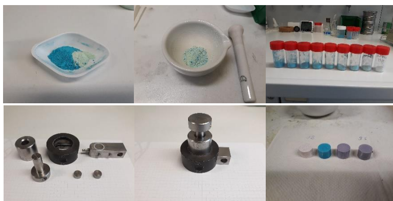
Fig. 5. Preparation of 13 mm pellets: Weighing, mixing, storing, pressing.
