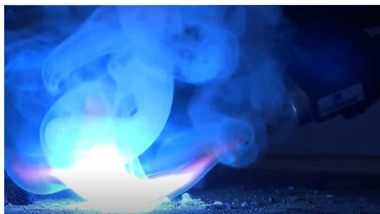
Fig. 2. A relatively dim blue flame appears above the burning surface of a 6 mm, 0.45 g blue firework star (pellet). Oxidizer: \text{KClO}_4 .
