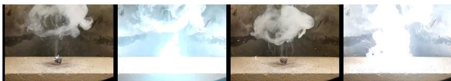
Fig. 3. Combustion process of a 8 mm white strobe pellet. Flash frequency: 6Hz. Composition: Ba(NO 3 ) 2 /KClO 4 /KNO 3 /MgAl (MX51 Eckerle)/GN/Polivinybutyral/NC/Cu (200mesh atomized) in ratio of 56.3/4.7/4.7/26.4/2.5/1/2.5/1.9 (Courtesy of P. Alenfelt).
