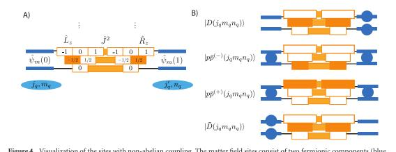
**Figure 4.** Visualization of the sites with non-abelian coupling. The matter field sites consist of two fermionic components (blue lines). The link is spanned up by two spin ladders *L* and *R*, which always have to have the same representation (spin length). (B) The three states, which are part of the ground state manifold.
