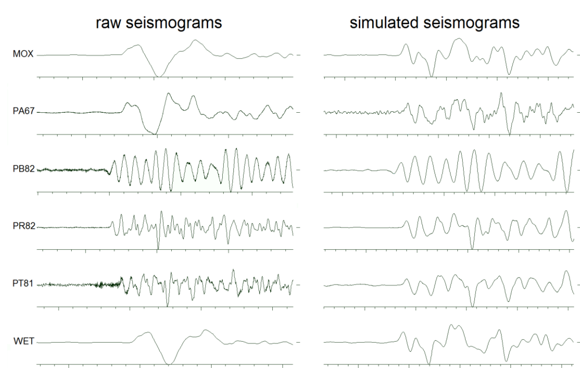
Fig. 3.3 Example of raw (left) and filtered with WWSS-SP filter (right) seismograms of EQ on 25.03.2007 at 00:41 UTC.
