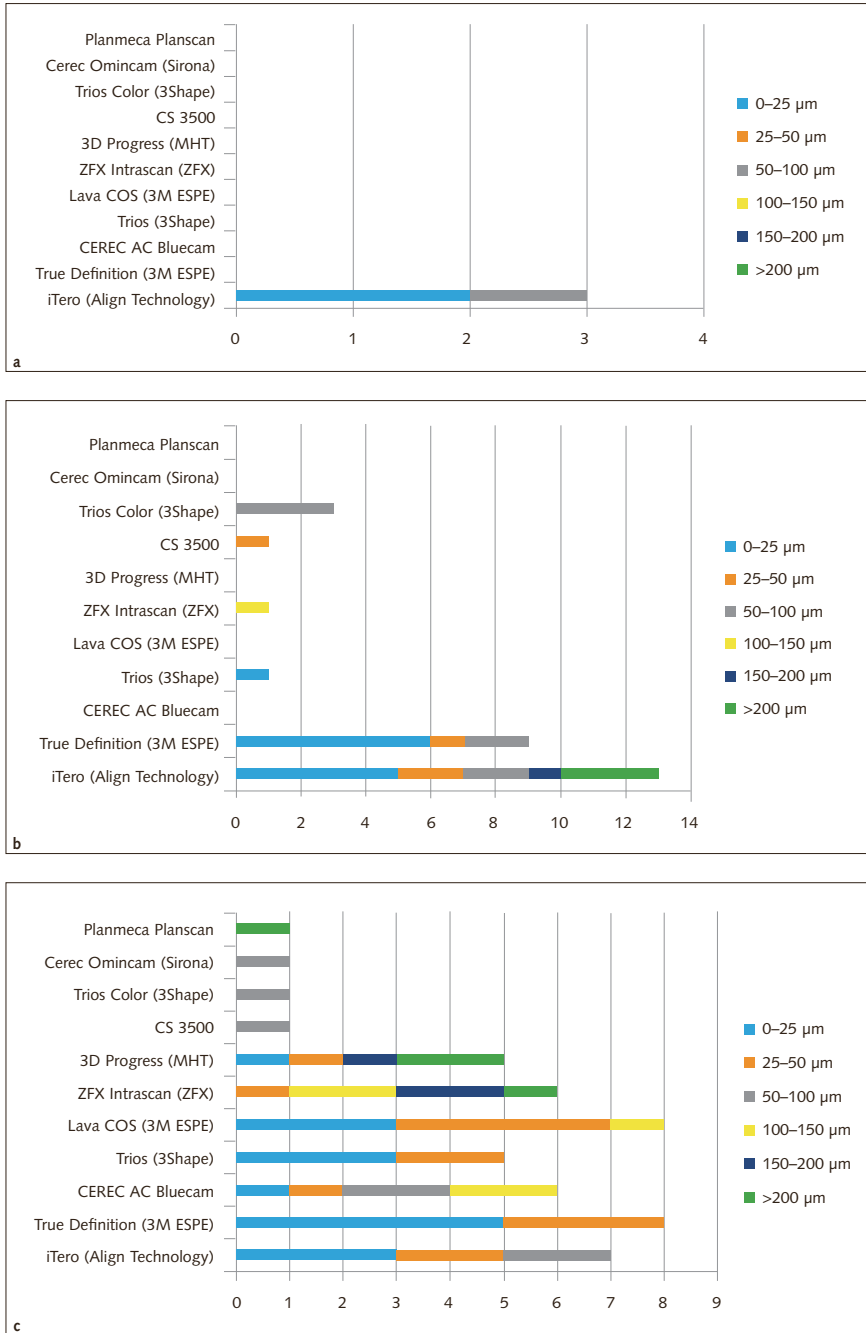
Fig 3 Digital implant impressions for: a) single-unit cases, b) FPD cases, c) fixed full-arch cases. Number of results reporting different linear absolute mean error intervals with certain IOS.
