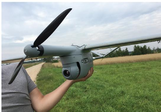
Figure 5. Fixed wing UAV “Buzzard”
