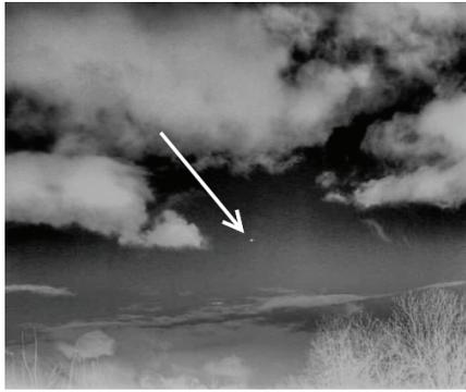
Figure 1. UAV at 200 m. detected by LWIR (long wave infra-red, 20 mm focal distance) camera at clear sky behind DJI Phantom 3
