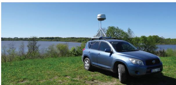
Figure 3. SIMRAD 4G<sup>TM</sup> radar mounted on SUV
