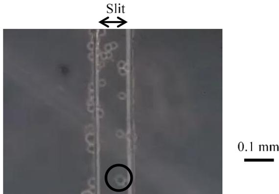
Figure 25. Cell (circle) passing through slit (length: 0.1 mm): flow from left to right [17].
