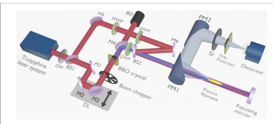
**Figure 7.** Experimental setup. DM, M1-M6: dielectric mirrors; HWP and QWP: half- and quarter-wave plates; BS1, BS2: beam splitters, PM1, PM2: parabolic off-axis mirrors; DL: optical delay line; BD: beam dump. SH and FH are shown by blue and red-pink color, respectively. THz radiation is represented by gray color.
