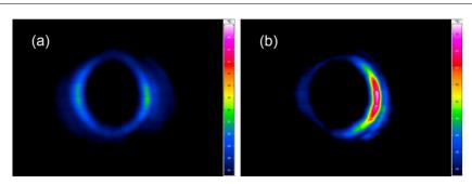
**Figure 9.** THz far-field beam patterns measured (a) at almost zero mutual FH and SH beam displacement and tilt and (b) for the beam displacement of about  $40~\mu m$  and tilt of about -0.7 mrad.
