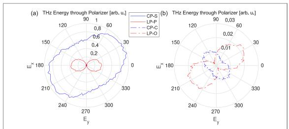
**Figure 8.** Experimental THz yield versus THz polarizer angle in arbitrary but comparable units. (a) CP-S (solid blue line) and LP-P (solid red line). (b) CP-C (dash-dotted blue line) and LP-O (dashed dotted red line). Energies of the FH and SH pulses were 0.92 and 0.03 mJ, respectively ( $r \approx 3.3\%$ ).
