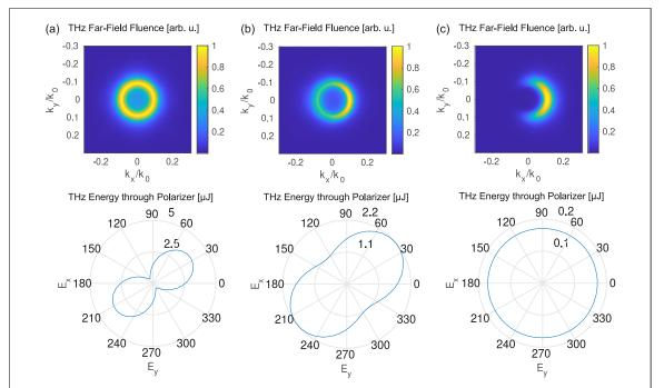
**Figure 11.** CP-S THz far-field fluence ( $\nu$  < 90 THz). (a) Perfect beam alignment. (b) SH beam displacement of about 4  $\mu$ m and tilt of about -0.04 mrad. (c) SH beam displacement of about 40  $\mu$ m and tilt of about -0.4 mrad.
