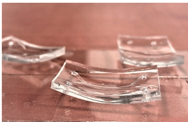
Figure 9. Deformation of PDMS chips in acetone and 4-methyl-2-pentanone.
