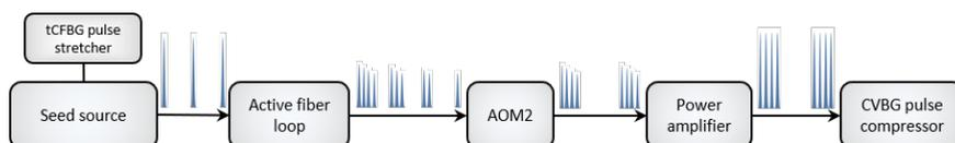
**Fig. 4.2.5.** Schematic diagram of the laser system synthesizing GHz bursts of equidistant ultrashort pulses. AOM2 - second acousto-optic modulator in the experimental setup, tCFBG - thermally tunable chirped fiber Bragg grating, CVBG - chirped volume Bragg grating. Adapted with permission from [A4].
