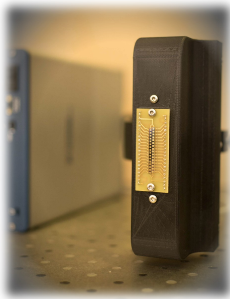
Figure 3. Photo of titanium-based microbolometer THz camera. It is composed of a linear array consisting of 2 lines with 16 pixels each. The left line is used for the detection of 700 GHz, and the right one for the detection of 300 GHz. It was realized via coupling of the sensors with antennas of relevant designs. The titanium bridge of 12 \mu\text{m} and 2 \mu\text{m} in length and width, respectively, was electrodeposited on the silicon nitride (SiN) membrane of 2- \mu\text{m} thick. The membrane was etched to reduce the heat capacitance and to increase the speed of operation. More details can be found in Refs. [188,190]. Courtesy of Laboratory for Microelectronics of Faculty of Electrical Engineering at University of Ljubljana and Luvitera Ltd, Vilnius, Lithuania. Photo: courtesy of Linas Minkevičius.
