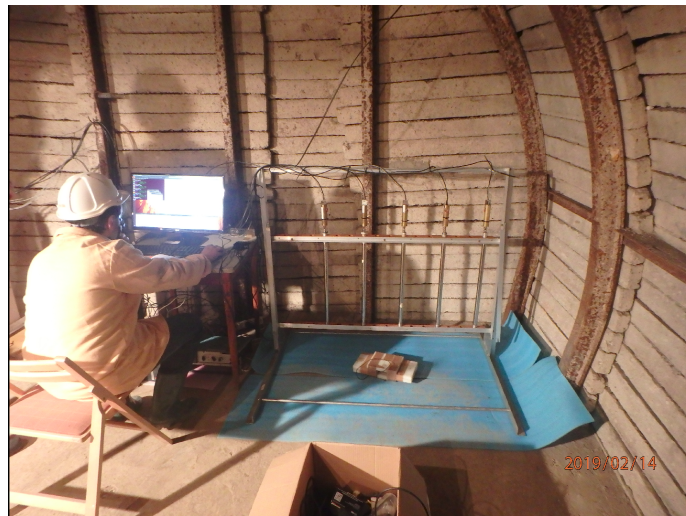
Figure 5: Measurements in the "Barbara" experimental mine. Five helium counters without a polyethylene cover are visible.
